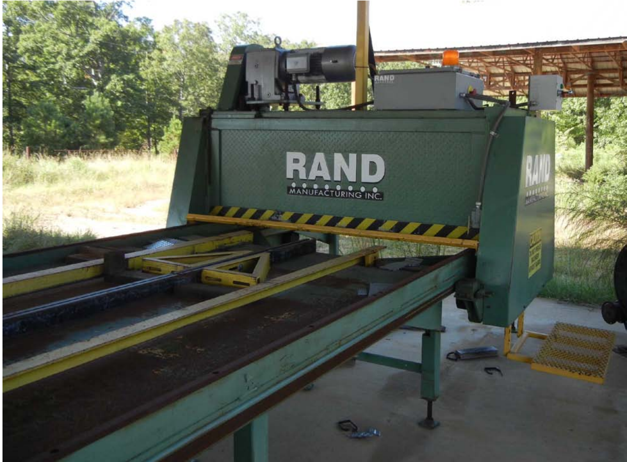
2007 RAND / AIR SET / FLOOR TRUSS GANTRY / MD-10-30-40 40' Roll Driven Floor Truss Machine / Builds 10" min to 30" max Deep Floor Trusses
